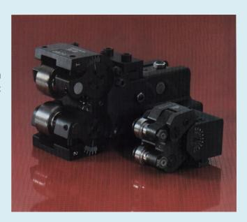
Reed attachments represent the fastest and most economic way to produce accurate thread rolling. It's possible to keep very tight tolerances even when producing very large quantities, the threads are much more resistant and downtime for the replacement of tools is reduced to the minimum while allowing a perfect repeatability.
