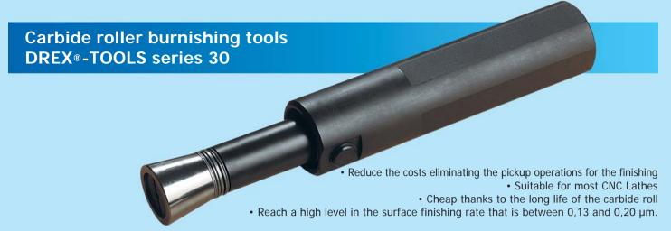
It is possible to burnish inside and outside diameters, fitting's radius or borders, shoulders and bar's end with only a single tool. **The carbide roller burnishing tools have been studied for being used on CNC lathes**. The surfaces to be burnish are prepared of turning with a roughness of 2-2,5  $\mu$ m. The tool, put in the due working position, has used with a speed same of the turning's speed, obtaining a roughness of 0,13-0,20  $\mu$ m. This replace the need of a pickup operation.
