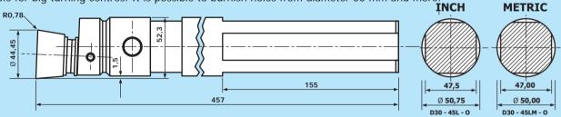
D30-45-0 This tool with a roll diameter 44,45 mm and a length of 305 mm has been studied for carrying out the burnishing on medium size holes. It is possible to burnish holes from diameter 50 mm and more.
