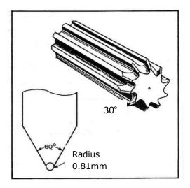
As a preliminary preparation to roller burnishing it's recommended to use a cutting tool with a radius of 0.8 mm. The head of the reamer should be sharpened to a lead angle of 30°. By using these parameters and advancing the cutting tool or reamer along the workpiece with a feed rate of 0.20 to 0.25 mm per revolution will create a surface with a roughness of 2.5 to 3.0  $\mu$ m ready to be roller burnished.
