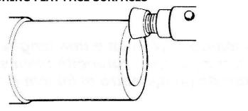
To establish the spring load when burnishing a flat face surface, advance the tool until it touches the workpiece's surface. After contact continue to feed at a rate of about 0.5 mm.. This will cause a light increase of the spring's load.
